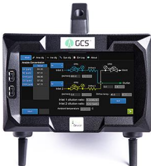
Figure 1 – ASDevices' intelligent Gas Calibration System (GCS) used for standard gas dilution
